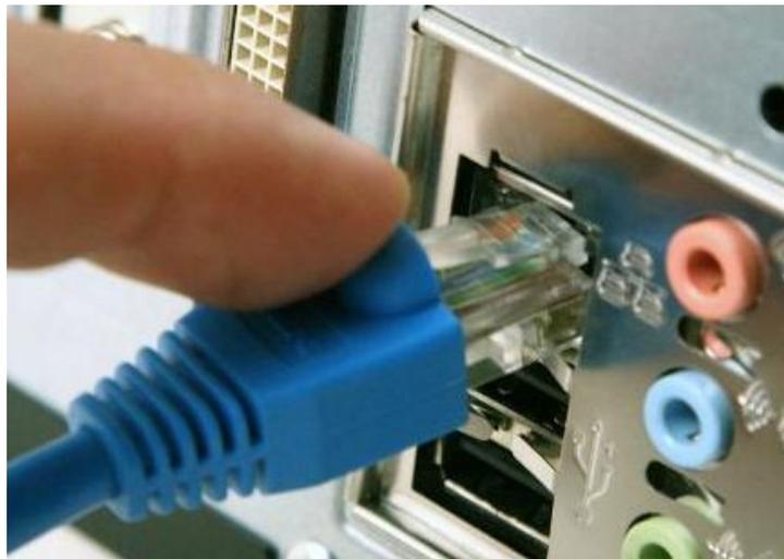
3. Connect the other end of the cable to the router. Afterward, connect the internet cable to the indicated port.
